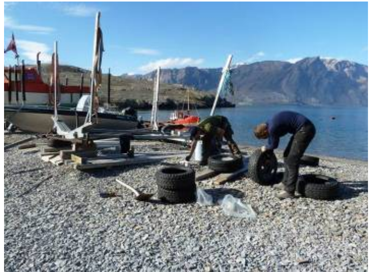
Renewing the old, rotten tires of "Agsut"s cradle.
